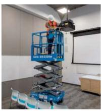
This scissor lift is equipped with an efficient, all-electric DC drive system that offers productive power for getting around indoor jobsites with quiet, zeroemissions operation. Heavy-duty and rental-ready, this new micro-sized scissor lift's top applications include construction in space restricted or congested locations, such as offices, high rise and retail spaces, as well as facility maintenance tasks.
