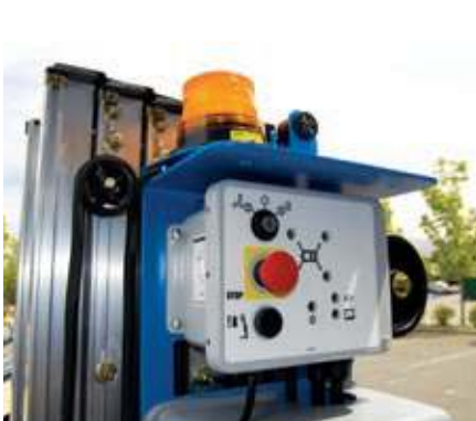
Operational Warning Light
