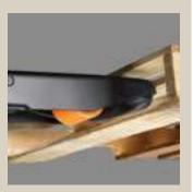
The smooth, rounded fork tips simplify pallet entry and are boxed in to add strength. In addition, the design of the fork tips prevents build up of debris.
