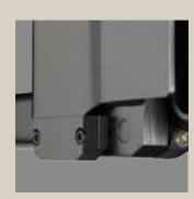
**Replaceable steel wear blocks** at the fork heels act as the first point of contact when underclearance is exceeded. This protects the undercarriage when driving over uneven surfaces, sharply angled dock plates or while operating on lift gates.
