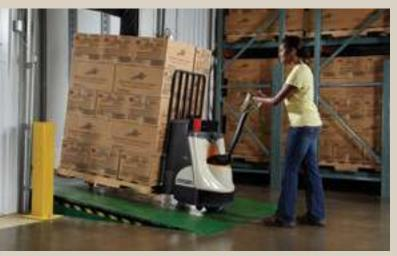
Crown's ramp hold improves operator confidence and control by minimizing the possibility of unexpected reverse travel when stopped on an incline. It also allows consistent speed on ramps, with or without a load.
