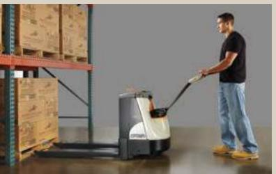
**Pallet entry** is enhanced by increased visibility of the fork tips resulting from the combination of a low profile power unit and Crown's exclusive fork tip indicators.
