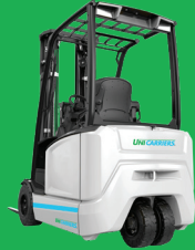
3-Wheel 2,700 - 4,000 lb Pneumatic MXST14-2 - MXS20-2 Built in: Finland
