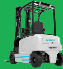
4-Wheel 3,000 - 4,000 lb Pneumatic MXS4-16 - MXS4-20L Built in: Finland
