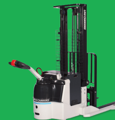
3,000 – 4,000 lb Walkie Straddle Stacker WSX30 - WSX40S Built in: Marengo, IL
