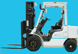
Small Diesel 4,000 – 7,000 lb Pneumatic PFD40M - PFD70M Built in: Houston, TX
