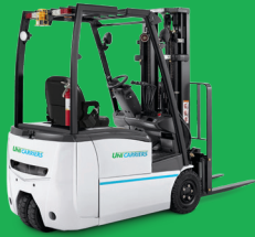
3-Wheel 3,000 – 4,000 lb Pneumatic TX30M - TX40M Built in: Houston, TX
