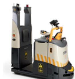
DualMode T 1000 Series Tow Tractor Rolling Load Capacity: 11000 lb
