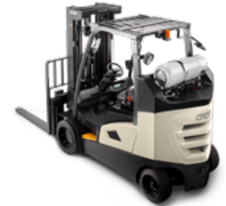
C-G Series, Models 35-55 Box Car Tire: Cushion Power: Internal Combustion - LPG Load Capacity: 8000 to 12000 lb Lift Height: 108 to 238 in
