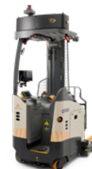
DualMode R 1000 Series Load Capacity: 3200 lb Lift Height: 183 to 400 in
