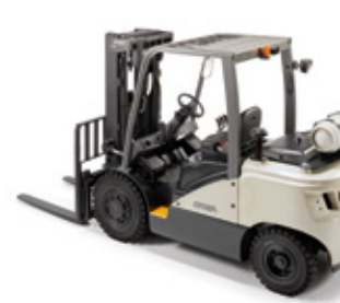
C-G Series, Models 35-55 Tire: Pneumatic Power: Internal Combustion - LPG Load Capacity: 8000 to 12000 lb Lift Height: 108 to 238 in
