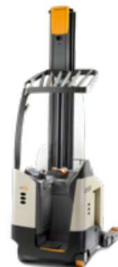
RM 6000 Series Load Capacity: 4500 lb Lift Height: 192 to 400 in
