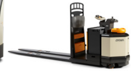
PC 4500 Series Center-Control Pallet Truck Load Capacity: 6000 & 8000 lb Forks: Double and triple lengths available
