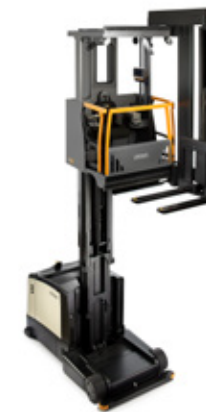
TSP 1000 Series (shown) Turret Order Picker Load Capacity: 3300 lb Lift Height: 193 to 531 in
