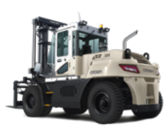
C-D Series, Models 100-160 Tire: Pneumatic Power: Internal Combustion - Diesel Load Capacity: 22000 to 36000 lb Lift Height: 118 to 256 in
