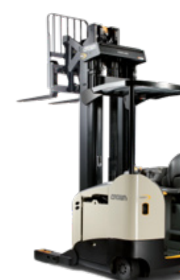
RR 5700S Series Load Capacity: 4500 lb Lift Height: 198 to 442 in
