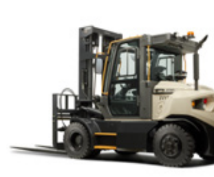
C-D Series, Models 60-90 Tire: Pneumatic Power: Internal Combustion - Diesel Load Capacity: 13500 to 20000 lb Lift Height: 118 to 256 in
