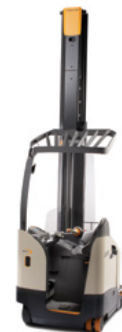
RM 6000S Series Load Capacity: 4500 lb Lift Height: 192 to 505 in
