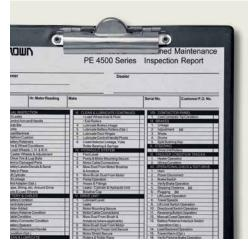
Crown technicians use truck-specific Planned Maintenance forms because recommended inspections vary for each type of truck.
