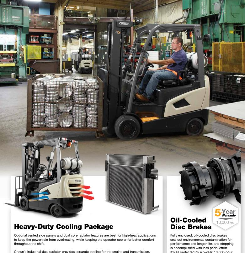
reducing fluid temperatures to protect and extend powertrain life. The optional heavy-duty cooling package is available for more demanding applications.
