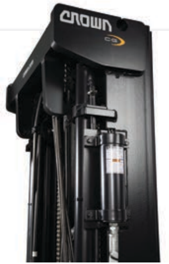
Optional Hydraulic Accumulator Reduces fork carriage bounce when traveling over uneven surfaces
