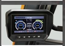
views of all the information the operator needs to know and more. Set PIN codes to quickly access truck settings such as speed limits, service intervals and vehicle diagnostics. A larger 7-inch display is
